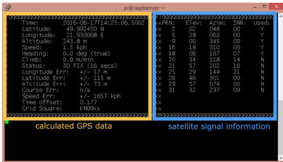
Figure 3. Display of position data obtained from GPS module
