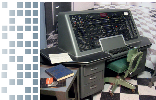
Konsola operatorska komputera UNIVAC I (UNIVersal Automatic Computer I)
